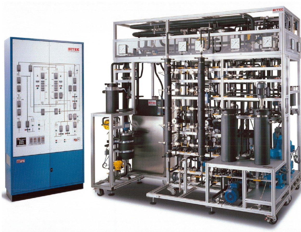
High-pressure pilot unit for ethynylation reactions (300 bar, 200 °C, 30 kg/h NH 3 /C 2 H 2 , 2 x 0.8 litre fixed bed reactors, fluid cyclone separator 2 litre).
