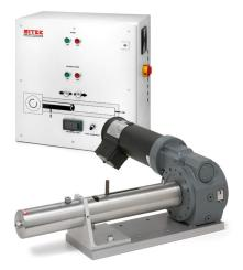
Electrical piston pump for pulsation-free flow generation. The control box includes a speed controller for the DC servo motor and allows an accurate control of the flow. Flow is adjusted using the potentiometer and is digitally indicated. Designed for manual and automatic operation mode.
