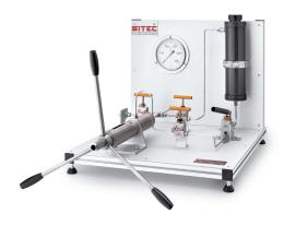
Pressure test system 2,000 bar (maximum pressure available 7,000 bar) allows the generation of high pressures by hand. The test sample can be connected to the bulkhead coupling.
