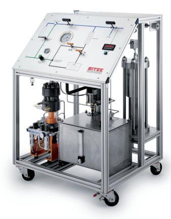
Pressure generation system 10,000 bar for gases (Austria). A pneumatically driven diaphragm gas compressor is used for prefilling to 1,000 bar. The intensifier driven by a hydraulic pump generates the pressure up to 10,000 bar. The actual pressure is digitally indicated.
